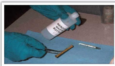
**Put Broken Instrument Glass Pieces Into A
